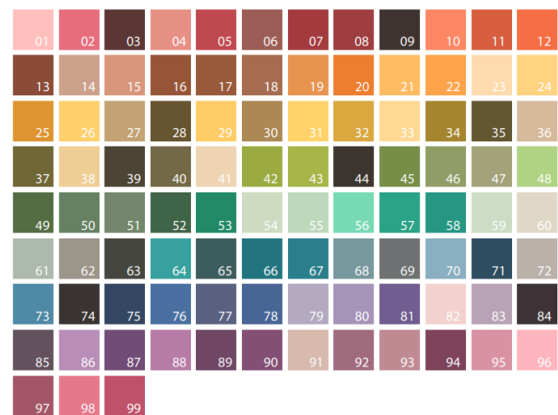
Figure 1. Colors of 99 samples used to calculate the color accuracy index, Rf, as approximately perceived under daylight illumination D50 (IES 2015, 2018; CIE 2017)
