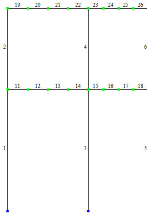
Figure 16.2 – General view of the frame after element addition
