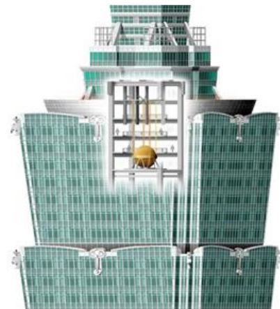
Figure 7.9 – Spherical damper in Taipei 101
