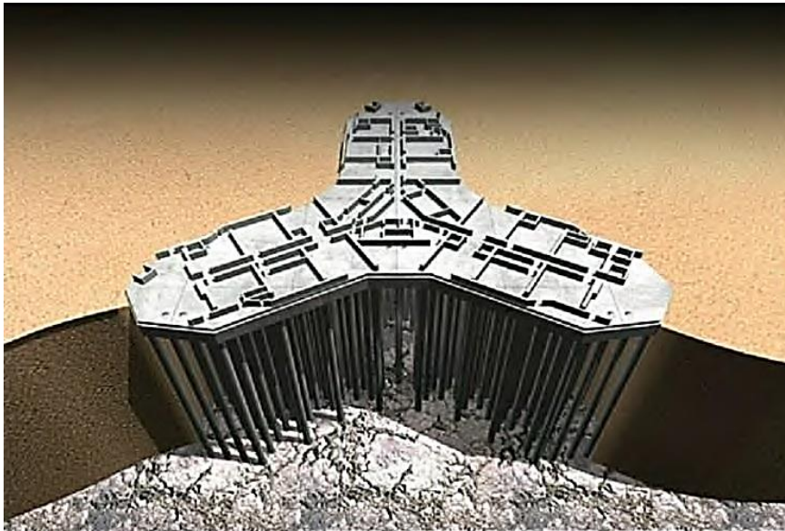
Figure 7.11 – Burj Khalifa Foundation Diagram
